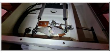
the water in and out. The rudder blade was supported by three brackets or bushings. The stock passed through the hull moulding via a GRP rudder tube with nylon bearing insert. The rudder was operated by wheel steering system which consisted of one steel helm wheel running a cable system attached to an aluminium quadrant clamped to the stock.
