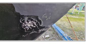
reduced before applying a new gelcoat layer. Proper drying is essential to prevent the trapping of moisture, which could exacerbate the problem over time. After the repair, it is advisable to conduct another moisture meter reading to confirm the effectiveness of the drying process.
